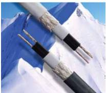
Heat Trace 2700 Series selfregulating heating cables can be cut and terminated in the field and safely overlapped without overheating or burnout. Their multilayered construction supplies a specified amount of heat at any point along their length in
