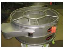
The Vibroscreen dewatering-clarifying screener separates solids from liquids on a batch or continuous basis. An imbalanced-weight gyratory motor affixed to the housing imparts vibration, which causes solid particles to move across the screen and exit
