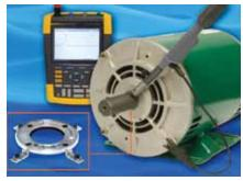
age test kit simplifies the measurement of induced voltages in variable frequency drives (VFDs), which helps reduce bearing damage and equipment downtime. The kit includes a replaceable probe tip that contains high-density conductive microfibers to ensure continuous contact with a rotating motor shaft and highly accurate voltage readings.
