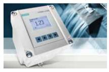
The Sitrans LUT400 series ultrasonic controllers have 1-mm measurement accuracy, and are available in three models: the LUT420 level controller; the LUT430 level, pump, and flow controller; and the LUT440 highaccuracy open channel monitor (which also provides advanced level, volume, and pump controls). They have backlit
