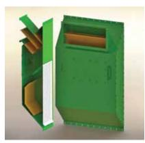
This spark arrestor for dust and fume collection systems channels sparks away from filters without the use of perforations or screens. It creates torturous paths that direct sparks and embers to a safe area, giving them more time to lose energy. The inlet transition is reversible, and provides horizontal or vertical entry without compromising control of the spark. The unit has a maximum capacity of 10,000 ft³/min, and contains an access door to allow debris to be removed. Camfil Farr APC
