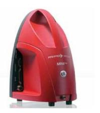
small leaks, and operates at working pressures up to 200 mbar with a detection limit of  $5 \times 10^{-7}$  mbar-L/s. It is equipped with two different leak detection functions. In the qualitative search mode, leaks can be quickly located. In the measuring mode, the size of the leak can be quantitatively determined. All measurement data can be saved in the device's remote-control system and stored on a USB stick for later use.
