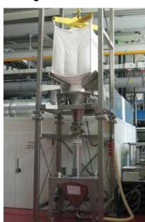
The BBUone is a bulk bag unloading station that optimizes dust-free material flow from the bag to a vacuum conveyor and downstream processes. It has a 2-ton capacity and a patentpending dust-tight connector to the feed hopper. The discharge chute connector contains product flow, and prevents dirt and other waste material that has collected on the underside of the bulk bag from contaminating the
