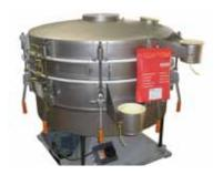
The Tumbler Screening Machine's (TSM) three-dimensional action maximizes product contact with the screen surface. It is suitable for fine and ultrafine screening, can have up to five
