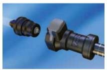
These quick-connect couplers are resistant to corrosion and acidic degradation as well as gamma sterilization. They are made of high-grade UV-resistant polypropylene, non-swelling Viton fluoroelastomer O-rings, and stainless steel springs, and have a pressure range of 0–100 psi and a temperature range of 32°F–160°F.
