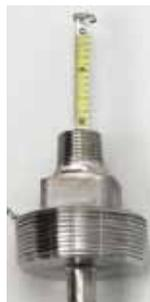
TL Series tape level indicators are designed to measure tank liquid levels in areas where electrical power is unavailable. The tape measure is sealed inside a liquid-tight stem, and a magnet around the stem floats on the surface of the liquid. The user determines the liquid level in the tank by sliding the tape out of the stem tube and reading the graduation mark when the magnetic interlock is felt. Three models are
