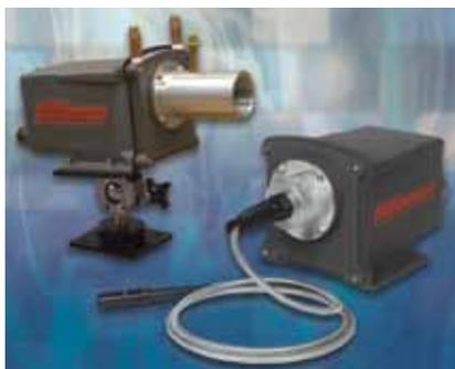
The Pro 100 and Pro 200 Series multiwavelength infrared temperature sensors operate in applications where thermocouples and resistance thermal devices (RTDs) are inaccurate, too slow, or too difficult to use. These sensors provide aim-and-read capabilities for non-graybody materials (*e.g.*, stainless steel, aluminum, brass, etc.) that are not accurately measured by single- or dual-wavelength sensors because the change in their emissivity
