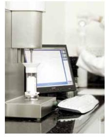
Powder Rheometer Software Version 5 has several new features and capabilities to support the FT4 Powder Rheometer for optimization of powderhandling processes. The FT4 measures the density, compressibility, and permeability of bulk solids to quantify powder properties in terms of flow and processability. Software Version 5 has an intuitive graphic interface that displays real-time test information, and provides step-by-step guidance to assist new users during test selection and execution.
