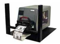
barcode verification, barcode validation, optical character recognition, optical character verification, field matching, and number/data validation. The software includes functions for automatic setup, job retrieval, and an alarm matrix with line and printer stop capabilities.
