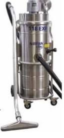
I, Group D and Class II, Groups E, F, and G environments. The vacuum is completely grounded, constructed of nonsparking Type 304 stainless steel, and equipped with conductive hose and accessories to eliminate static charge. It features a 13.2-gal
