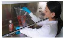
The FlexFill assembly enables singleuse biocontainer transfer. It provides a convenient way to aseptically transfer small bottled volumes of cell culture media, sera, reagents, supplements, buffers, and microcarriers to a bioreactor. It is delivered sterile, and is available in volumes from 500 mL to 6 L. Assemblies can be customized to support aseptic connectivity with a host of fitting and tubing options to allow for a seamless integration with the process.
