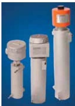
DFX Series heater elements are isolated from the fluid flow path. The heater elements and a coiled, seamless, Type 316 stainless steel flow tube are embedded in a lightweight aluminum casting. This design is said to be ideal for heating deionized water, solvents, sterilization gases, and other substances that are prone to contamination.
