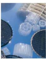
The AnoxKaldnes moving-bed biofilm reactor (MBBR) uses biofilm carrier elements to provide optimal conditions for complete biological treatment or pretreatment in a variety of chemical industry wastewater treatment applications. The process removes biochemical oxygen demand (BOD), chemical oxygen demand (COD), nitrogen, and phosphorous in compact, robust, reliable systems
