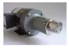
The G3000 and G4000 series gear pumps in Hastelloy C276 can handle chemicals that cannot be tolerated by 316 SS, and pressures and temperatures for which plastic pumps are unsuitable. They can be close-coupled to variable-speed motors for accurate, pulseless metering. Non-lubricating, low-viscosity liquids can be handled by models with an alloyagainst-plastic-gear construction.
