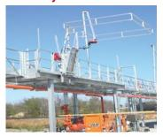
Track mounted gangway can be moved back and forth along the elevated track and extended as necessary to provide safe and easy access or egress from the vehicle no matter what the spotting or configuration.
