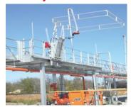
Track mounted gangway can be moved back and forth along the elevated track and extended as necessary to provide safe and easy access or egress from the vehicle no matter what the spotting or configuration.
