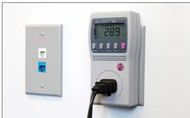
■ Figure 1. The Kill A Watt meter is an easy-to-use tool to measure the power consumption of plug-in appliances. Photo courtesy of P3 International.
