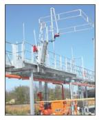
Track mounted gangway can be moved back and forth along the elevated track and extended as necessary to provide safe and easy access or egress from the vehicle no matter what the spotting or configuration.
