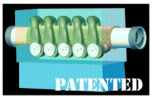
Cross Flow Rotary<sup>TM</sup>; PATENTED Coarse, free-flowing material (e.g. catalysts, ceramics, etc.) can be heated and reacted with a through-flowing gas. Locally, gas flows perpendicular to the solid material path. Globally, the gas can flow counter current yielding very high energy efficiency.
