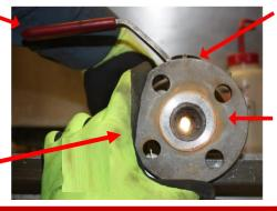
Valve handle failed and allowed handle to turn without closing the valve
