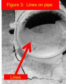
thicker piece of pipe to the designed profile. The investigation team asked an experienced machinist to inspect the failed pipe. The machinist immediately recognized that the lines were not signs of erosion, but actually tool marks from a boring tool. When the pipe was bored, the tool had not been inserted properly, but off-center. This resulted in the pipe being only about 25% of the intended thickness at the top, and consequently weakened.
