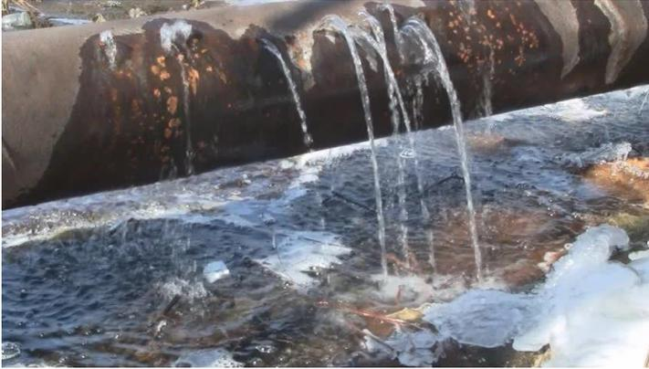
A company decided to stop making a chemical product. One of the input materials was toxic and corrosive phosphorus trichloride ( $\text{PCl}_3$ ). The lines to the storage tank and the process area were cleared of  $\text{PCl}_3$ . A few years later, an operator found a leak outdoors. The investigation found that the leak was coming from the “empty”  $\text{PCl}_3$  line. No one was injured and the spill was contained.
