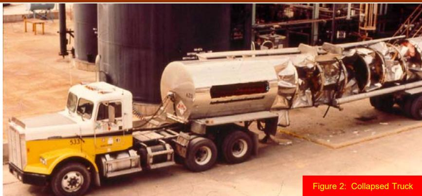
Figure 2: Collapsed Truck
