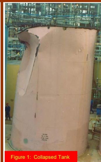
Figure 1: Collapsed Tank
