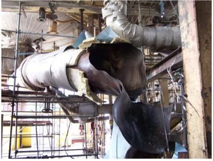
indicated that the reaction resembled closely the decomposition of TNT explosive. Fortunately, nobody was injured. The incident showed that it was critical to avoid leaks of the nitrate salt, to detect leaks if they did occur, and to have a safe shutdown procedure if there was a leak.
