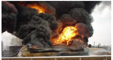
a dozen employees were hospitalized and there was significant property damage. The incident investigation found that the tank was being filled and, unknown to the operators, the tank level gauge AND the high level alarm had failed. The operators did not monitor the filling operation closely because they believed that the tank still had plenty of capacity.
