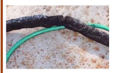
After twenty-two 30-pound hand-held chemical fire extinguishers, two 125-pound wheeled fire extinguisher units, and the firewater system were used, the fires on both decks were contained. One man received second-degree burns. After the fires were extinguished, it was discovered that the hose used to feed methanol from the transporter to the storage tank was split and had been repaired with duct tape prior to the operation!
