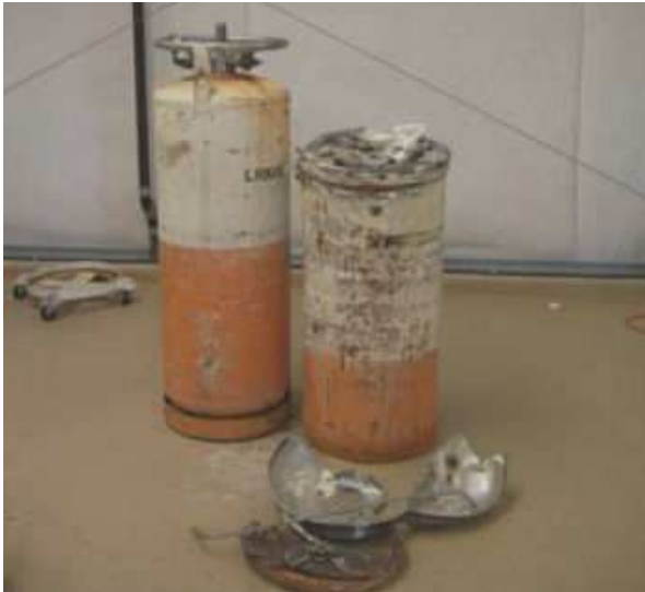
Intact cylinder and remains of ruptured cylinder
