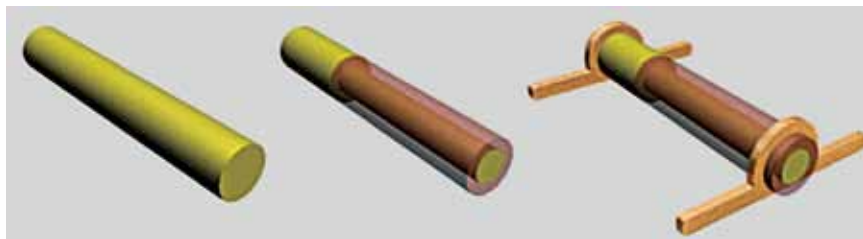
▲ The solar nanowires are made by first dipping a CdS nanowire (green) into a solution of CuCl, where cation exchange creates a Cu 2 S shell coating (brown). Metal contacts are then deposited on the CdS core and Cu 2 S shell. Image courtesy of Yang, et al.
