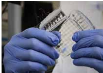
▲ Lines of carbon nanotubes intersect to form a grid of tiny parallel-plate capacitors. Because the capacitance of a parallel-plate capacitor is inversely proportional to the distance between the plates, when the grid is compressed, its capacitance increases. Image courtesy of Steve Fyffe, Stanford News Service.
