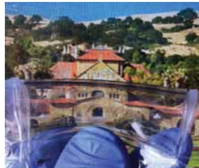
▲ The transparent, stretchable pressure sensor maintains its conductivity when stretched up to 2.5 times its original length. Image courtesy of Steve Fyffe, Stanford News Service.
