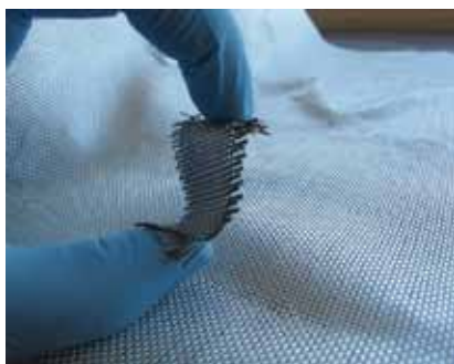
▲ A natural fibrous material is shown here with (small swatch) and without the conductive coating. Adding electronic functionality to fabric systems is important for new applications in healthcare and environmental monitoring. Photo courtesy of Jesse Jur and Gregory Parsons, North Carolina State Univ.
