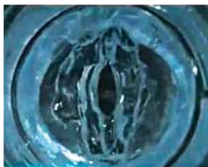
▲ This snapshot is from a high-speed video recording that documented a sample of PEG gel vibrating in response to voice-like airflow. Image courtesy of MIT and MGH. (The video is available at www.youtube.com/watch?v=10JAW0K1RTs .)
