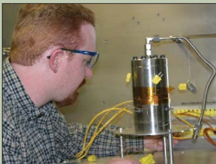
Sandia National Laboratories engineer Mark Zimmerman integrates a hydride bed with temperature sensors.
