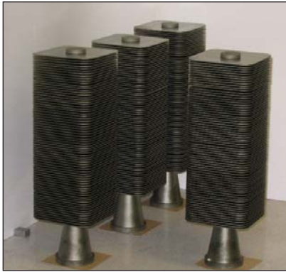
■ Figure 1. The Air Products' ITM Oxygen system uses stacks of ceramic wafers, which separate oxygen from hot, compressed inlet air, as a cost-effective alternative to conventional cryogenic distillation. Credit: Air Products and Chemicals.
