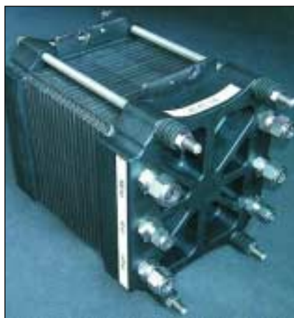
Figure 3. Ticona's prototype proton-exchange membrane fuel cell, designed with injection-molded bipolar plates, reduces the production cost of this model by 50%.
