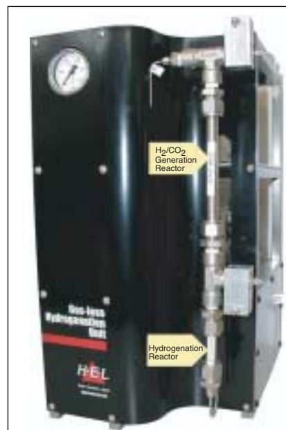
Figure 1. HEL Group’s supercritical flow reactor measures 35 cm wide, 30 cm deep, and 50 cm high and handles gas flowrates up to 10 g/min.
