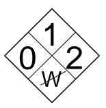
The area with a "0" in the diamond denotes health hazard, the area with the "1" denotes fire hazard and the area with a "2" denotes reactivity hazards. The box at the bottom is used to denote special hazards, e.g. incompatible with water.
