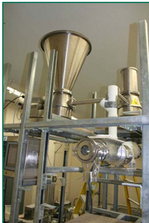
Figure 3 – Development of Wet Granulation processes to convert batch powder processing units to continuous powder processing systems – Rutgers University
