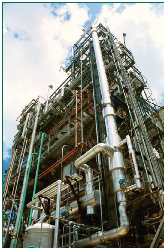
Figure 1 – Dividing Wall Column Pilot Plant at The University of Texas at Austin
