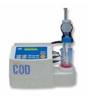
holder simplifies electrode mounting and dismounting, allowing smoother operation. A countdown timer and bell let the user know the status of the oxidation. The analyzer is able to handle coulometric titration with colored samples. A secondary differential helps to detect the titration endpoint, which results in more-precise measurements. Features like an easy-to-read control panel, touch-key input, and dialog interface make the analyzer easy to use.
