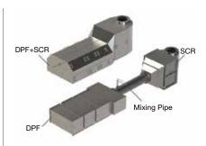
continuously combust the soot that is collected on the DPF, with selective catalytic reduction (SCR). Engine exhaust flows first through the CRT for PM, CO, and HC removal. Urea is then injected into the exhaust before it enters the SCR catalyst module, where NOx is reduced.
