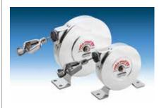
New additions to the Rota-Reel line of static grounding reels include the Rota-Reel 200-20R-ST and the Rota-Reel 700-50R-ST, which have cable lengths of 20 ft and 50 ft, respectively. The reels' exterior is constructed of Type 304 stainless steel, which is generally acceptable for use in hazardous (explosive) environments because of its low sparking tendency. This material also offers corrosion resistance, and is appropriate for applications where paints and coatings
