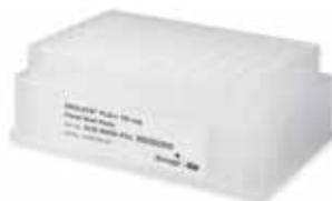
The Isolute PLD+ plate is designed for the cleanup of blood-based matrix samples for analysis by liquid chromatography-tandem mass spectrometry (LC-MS/MS). It incorporates a phospholipid-scavenging sorbent layer, which removes phospholipids from the sample during the filtration step. Isolute PLD+ plates remove more than 99% of plasma proteins and phospholipids — producing cleaner extracts for a broad range of analytes. Once puri-
