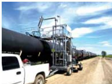
hoses and loading arms to transfer products from one vehicle to another. The platform can be designed for double-sided operation for maximum flexibility, and can be customized to allow access to two rolling vehicles simultaneously. Available accessories include a trailer package, loading arms, hose handlers, pump and metering systems, electrical grounding, lighting packages, and safety showers, among others.
