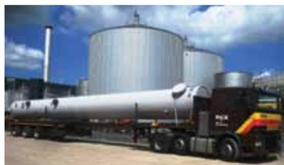
This external-circulation sludge bed (ECSB) is a high-flowrate granular sludge-bed reactor system that is suitable for treating industrial wastewater streams containing biodegradable material. The anaerobic treatment technology is robust and has no odor emis-
