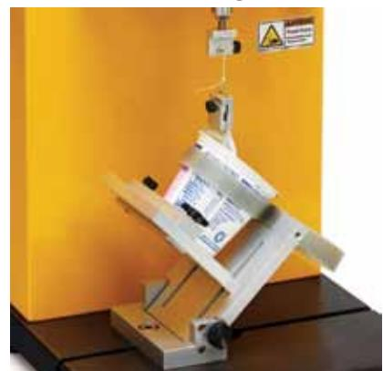
The TA-GPJ general peeling jig was developed to measure the force required to peel the lid off a sealed container. A strong adhesive bond is critical to prevent contamination and spoilage, but ease and consistency of opening are equally important to consumers. The TA-GPJ can be adjusted to remove the lid at 0-deg., 45-deg., or 90-deg. angles. It is suitable for measuring lid strength for products in the pharmaceutical and food and beverage industries.
