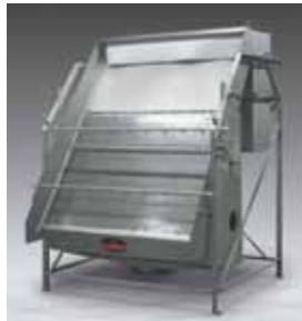
The Cross-Flo static dewatering sieve continuously removes solids from waste streams at ultrahigh rates, which facilitates clarification and dewatering of slurries. The screening deck is fitted with a stainless steel wire screen that has slots oriented perpendicular to the flow of material. An extended acceleration/orientation ramp in the upper por-
