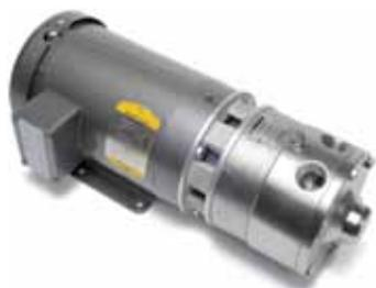
Because the stainless steel, magnetic-drive Coro-Flo MDC pump has no mechanical seals, maintenance requirements are significantly reduced. Sealless technology offers maximum protection when handling corrosive and toxic chemicals, because it prevents emissions to the atmosphere. The pump has a close-coupled design that makes installation quick and easy. Its stainless steel construction is well-suited for highly corrosive applications.
