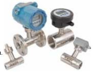
mounted on a bearing and pin assembly. The rotational speed of the impeller is measured by a magnetic pickup housed in the probe assembly. The meter housings are constructed of corrosion-resistant stainless steel. The meters can be customized to handle a variety of flow ranges and pressures, with threaded or flanged connections, and various display requirements. In addition, the user can specify a temperature rating up to 120°C, 230°C, or 350°C.
