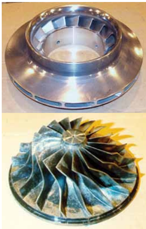
▲ Figure 5. Impellers can be either shrouded (top) or open (bottom).
