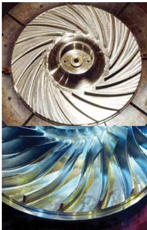
▲ Figure 6. Impeller blades can be either two-dimensional (top) or three-dimensional (bottom). The 2D blades in the top image have a circular arc shape, whereas the blades in the lower image have a complex 3D shape.
