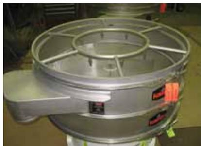
The Vibroscreen dewatering-clarifying screener separates solids from liquids on a batch or continuous basis. An imbalanced-weight gyratory motor affixed to the housing imparts vibration, which causes solid particles to move across the screen and exit
