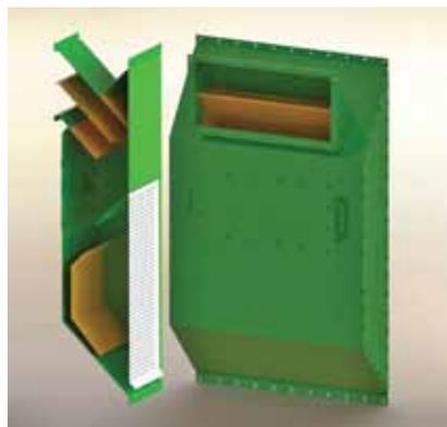
This spark arrestor for dust and fume collection systems channels sparks away from filters without the use of perforations or screens. It creates torturous paths that direct sparks and embers to a safe area, giving them more time to lose energy. The inlet transition is reversible, and provides horizontal or vertical entry without compromising control of the spark. The unit has a maximum capacity of 10,000 ft<sup>3</sup>/min, and contains an access door to allow debris to be removed.
