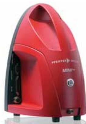
small leaks, and operates at working pressures up to 200 mbar with a detection limit of  $5 \times 10^{-7}$  mbar-L/s. It is equipped with two different leak detection functions. In the qualitative search mode, leaks can be quickly located. In the measuring mode, the size of the leak can be quantitatively determined. All measurement data can be saved in the device's remote-control system and stored on a USB stick for later use.
