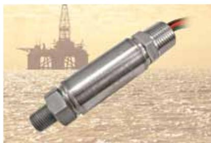
The AST46SW explosionproof pressure switch has a single-pull, double-throw configuration with factory-set switch points. Its one-piece stainless-steel sensing element can measure pressure in the most extreme temperature conditions. The switch has an operating range up to 20,000 psi, and can maintain high performance with zero signal drift due to its thick and robust sensing diaphragm. The
