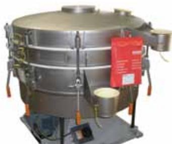
The Tumbler Screening Machine's (TSM) three-dimensional action maximizes product contact with the screen surface. It is suitable for fine and ultrafine screening, can have up to five
