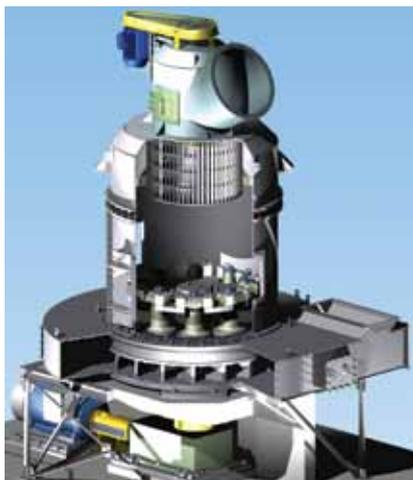
The Raymond 120-in. roller mill system is able to dry, pulverize, classify, and deliver granular to fine particles. It can handle feed particle sizes of 10–70 mm, and is suitable for materials that are classified as 5 or less on the Mohs scale of hardness. The roller mill controls product size and quality using a minimum amount of power. Additional features include journal assembly, vertical shaft hub connection, and fabricated plow support.
