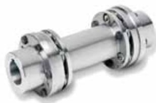
The Dodge Disc coupling is suitable for pumping applications in the oil and gas industry. Its disc geometry minimizes stress during operation, which results in high torque ratings and long lifespan. The disc coupling has no relative movement between mating surfaces, and therefore does not need lubrication during operation. A large-hub option increases the maximum bore capacity in applications where the coupling size is determined by the shaft diameter rather than the torque requirement.
