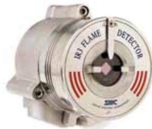
The 3600-I Triple IR flame detector can detect fuel and gas fires at long distances with very few false alarms. It features a heated window to eliminate condensation and icing, a compact design, and low power requirements. The flame detector has an automatic and a manual built-in-test (BIT) to assure continued reliable operation. Output options include relays for alarm, fault, and auxiliary; 0.2 mA (stepped); HART protocol; and RS-485 (modbus compatible).
