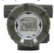
Loop-powered indicators provide a local display of a sensor's measured value. The MLX loop-powered indicator operates from a 4–20-mA DC input, and its NEMA 4X aluminum housing meets Factory Mutual (FM) explosionproof requirements. It includes a six-digit numerical LCD display, a six-digit alphanumeric display for engineering units, and a 20-segment bar graph that indicates 0–100% of full scale. Stainless steel tags and epoxy resin or polyurethaneepoxy paint coatings are available.
