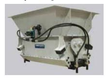
The Vibra-Gate valve uses vibration to dislodge materials, and can be used to control feed rates during filling operations. It moves stored granular material without the need for flushing, and is suitable for discharging sticky, cohesive, and high-moisture materials from bins and hoppers.
