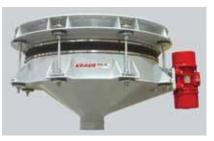
The GYRO EX bin-activating discharger/feeder produces a controlled gyratory motion to withdraw granular materials from bins, storage silos, and hoppers at any desired feed rate. It uses radial force to create a uniform circular motion on both the upper activation cone and the lower discharge cone. Because the material load is completely supported by the upper cone, product is not compacted within the lower cone. This, coupled with the steep angle of the discharge cone, prevents ratholing.
