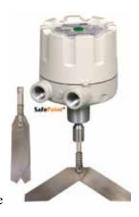
the outside of a bin or silo through a 1-1/4-in. NPT or 1-1/2-in. BSPT coupling. A spring-action feature allows the paddle to be removed, if necessary.
