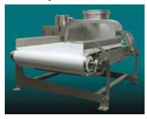
The sanitary DEA open-frame weighbelt feeder provides weight-controlled feeding and weight indication for fragile materials such as cereals, snack foods, and pasta. It features Type 316 stainless steel product-contact surfaces, and is offered in 12-in. and 24-in. belt widths with belt-weight influence compensation (BIC) to accommodate feed rates up to
