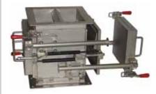
These vertical spout magnets separate fine to large ferrous contaminants from high-volume, gravity-fed product streams. Tramp metal is removed from moist, lumpy, granular, and powdered products by two powerful opposing magnets mounted on the outside of the housing. A center diverter on the housing inlet helps direct product toward the magnets. The system's single trapface design ensures that tramp metal is not washed back into the product stream before it is discarded into collection trays.
