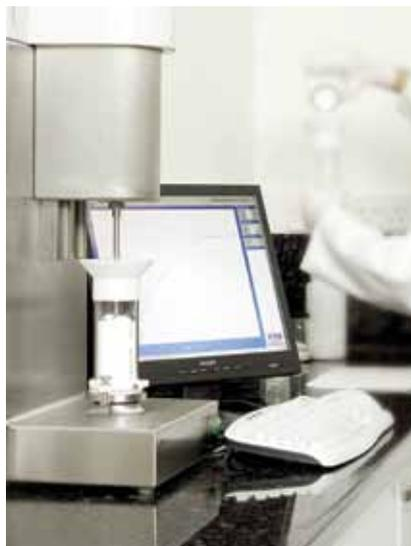
Powder Rheometer Software Version 5 has several new features and capabilities to support the FT4 Powder Rheometer for optimization of powder-handling processes. The FT4 measures the density, compressibility, and permeability of bulk solids to quantify powder properties in terms of flow and processability. Software Version 5 has an intuitive graphic interface that displays real-time test information, and provides step-by-step guidance to assist new users during test selection and execution.
