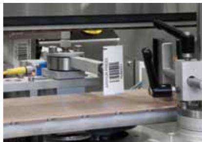
The Model 277 Autosert outsert applicator attaches outserts to round, square, or rectangular pharmaceutical containers at high speeds. It handles outserts with dimensions of 0.875–2.5 in. (22–63 mm) wide by 1.125–4 in. (29–100 mm) high and up to 1.5 in. (38 mm) thick, at speeds up to 220 bottles/min. It uses hot-melt glue adhesion to secure heavy outserts.
