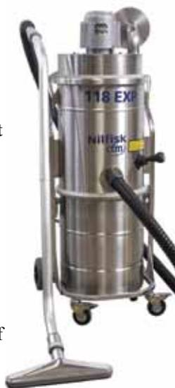
I, Group D and Class II, Groups E, F, and G environments. The vacuum is completely grounded, constructed of nonsparking Type 304 stainless steel, and equipped with conductive hose and accessories to eliminate static charge. It features a 13.2-gal
