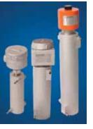
DFX Series heater elements are isolated from the fluid flow path. The heater elements and a coiled, seamless, Type 316 stainless steel flow tube are embedded in a lightweight aluminum casting. This design is said to be ideal for heating deionized water, solvents, sterilization gases, and other substances that are prone to contamination.
